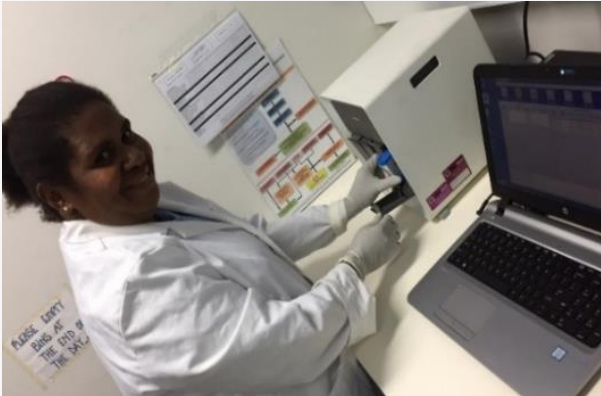
Use of GeneXpert instrument to diagnose and detect the DNA specific to M. tuberculosis complex and resistance to rifampicin.
